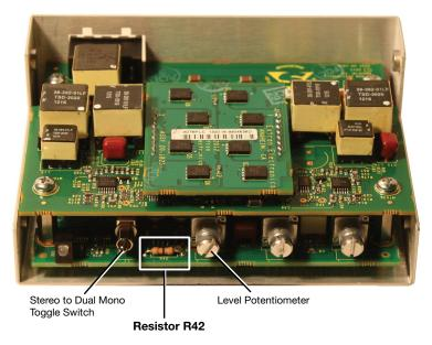
Figure 10. Front View, Showing the Location of Resistor R42
